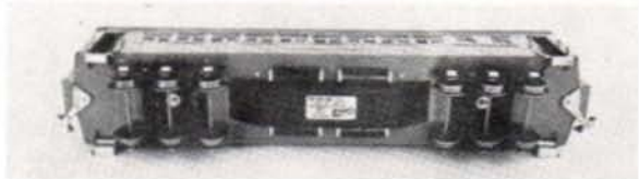
A BOTTOM VIEW - SHOWING BELLY PAN WITH FOUR AIR TANKS, SIX WHEEL TRUCKS WITH ROLLER CURRENT PICK UP FOR INTERIOR LIGHTS, AND AUTOMATIC COUPLERS.
