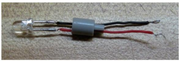
Straighten out the black and red leads and thread them through the 2 holes in the grey LED base.
