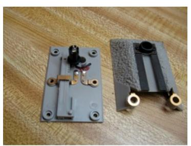
Remove the four remaining screws from the switch stand and separate the two halves.
