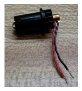
Bring both wires out through **ONE** slot in the brass bushing.
