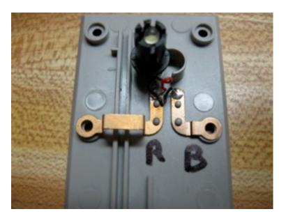
Note the position of the black and red wires on the switch stand base.
