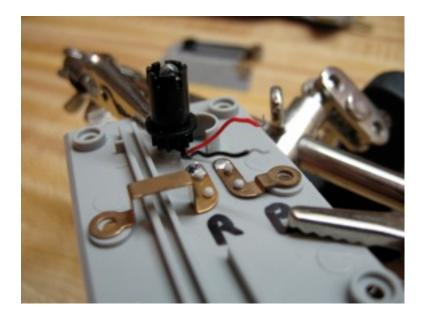
Now heat the two solder joints and pull the wires off of the solder pads.
