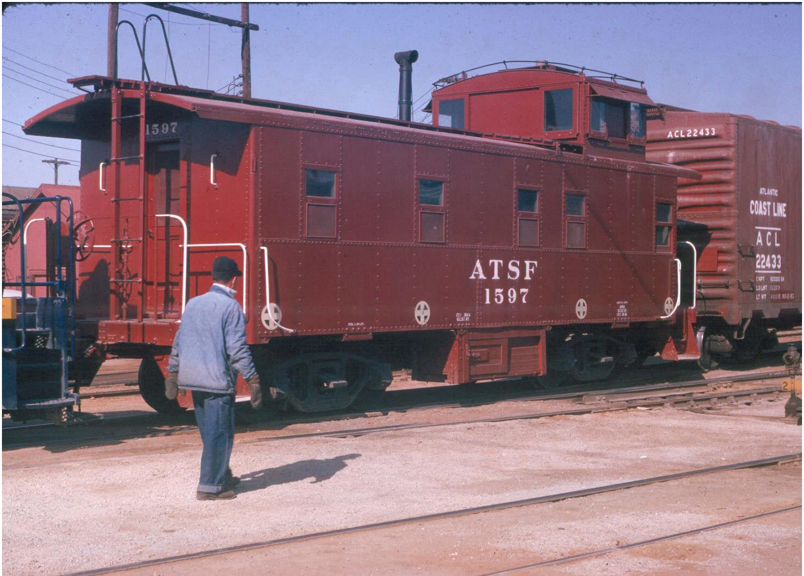
1597 on GC&SF radio equipped – can antenna
