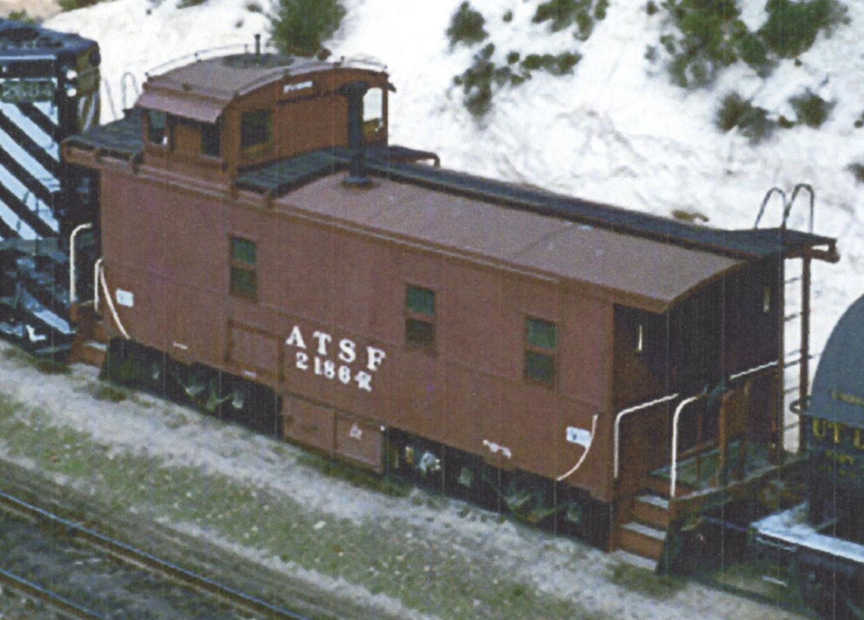
2186 R radio equipped -wagon wheel antenna Note the black running boards and platforms boards
