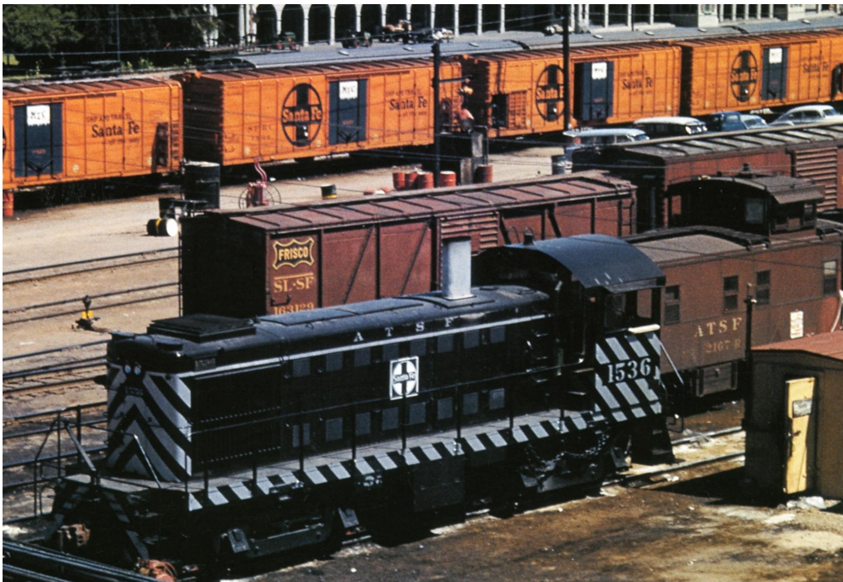
Barstow October 1961 can antennas used on 1536 and caboose 2107 R J. Mica photo SFRH&MS Warbonnet
