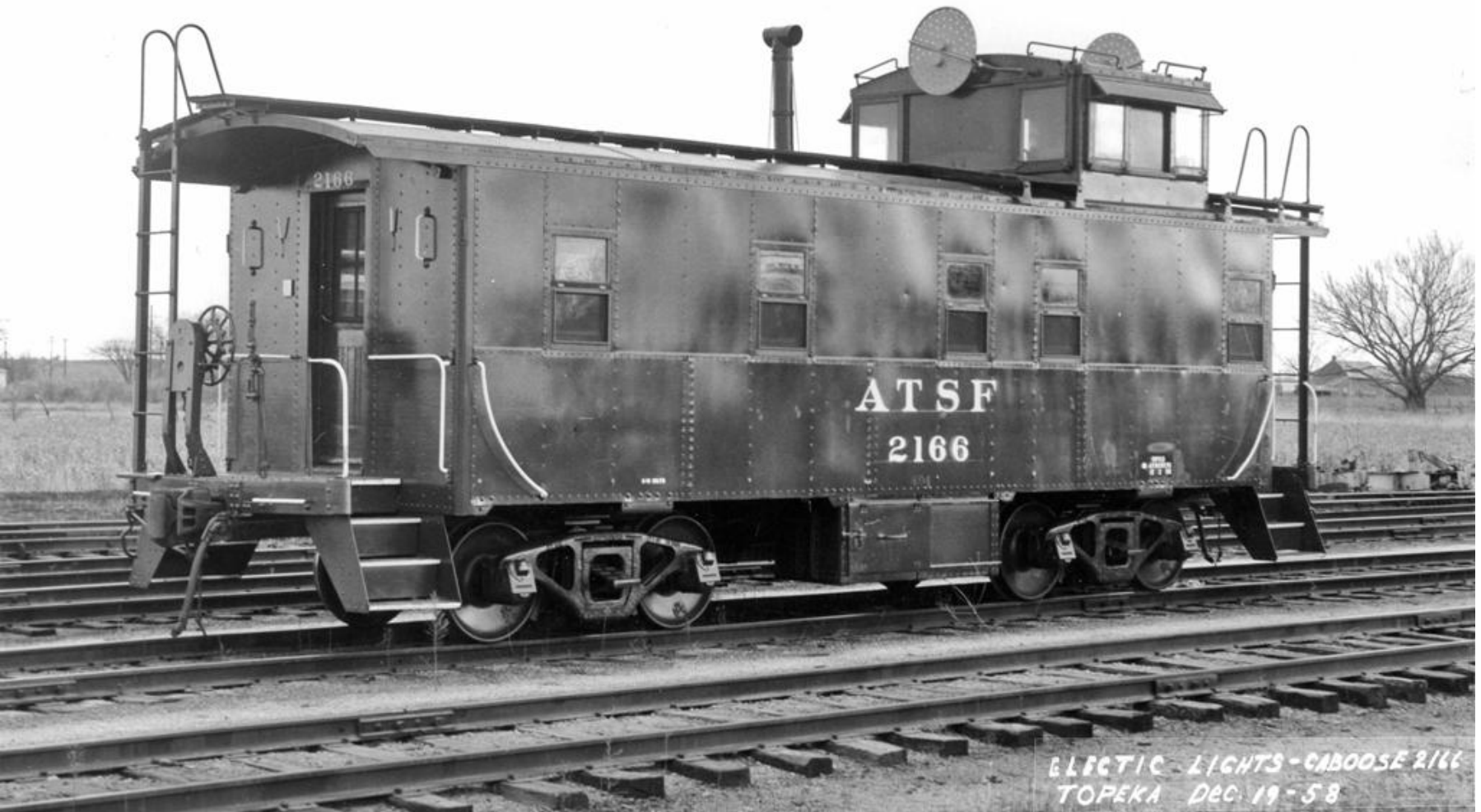
Caboose Cars Equipped with Electric Lights to Comply with Colorado Law - Job 414 (22 cars).
