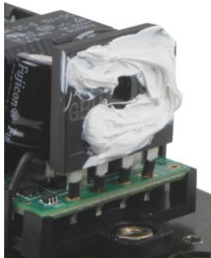
Apply white thermally conductive grease to bridge rectifier & the mounting spot for the metal heat sink bracket.
