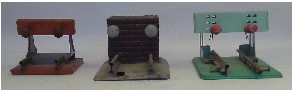
The last three are a bit messy; the left is marked Germany and looks as though it can bear no shock. The middle is a Bing buffer. The right is applicable for multiple gauges; also the buffer width and height can be adjusted on a rickety way.
