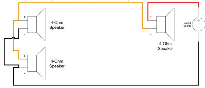
4-Ohm Series-Parallel Connecton for A-B-B-A Speakers in All Units Net Impedance = 4 Ohms (allows lead A/B pair to run with slave A/B pair)
