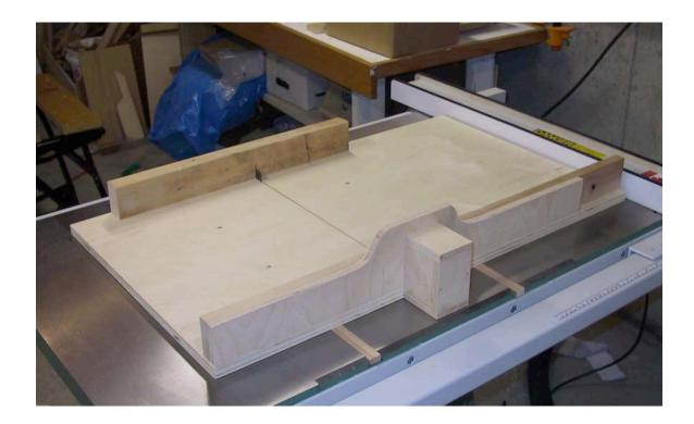
The fence at the base of the saw is last thing to be attached. Initially two screws attach the fence to the platform, one placed at either end of the fence and driven into the fence from below the platform. One of the screws becomes a pivot point for adjusting the fence square to the cut. The other screw is eventually removed and relocated to set the fence in the square position.
