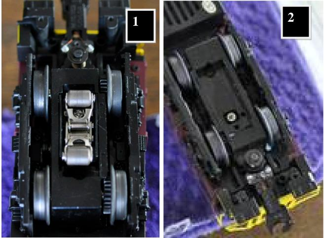
MTH RS-3 Pickup Roller Binding Fix Prevents engine from stalling or "bouncing" on uncoupler track magnet
