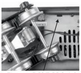
in DCC you must install a DCS-DCC switch. If Figure 7: DCS/DCC Switch you operate in DCS or conventional mode, it is not necessary to install the DCS/DCC Switch. Please refer to the "Modes of Operation" section to see and learn about the differences in the various operating modes.
