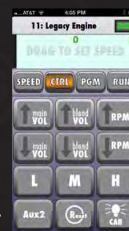
RIGHT: Use a combination of both main and blend volumes to set overall volume and the balance between foreground and background sounds. RPM up and down change the run level of diesel prime movers. On a steam engine, these buttons become Labor up/down.
