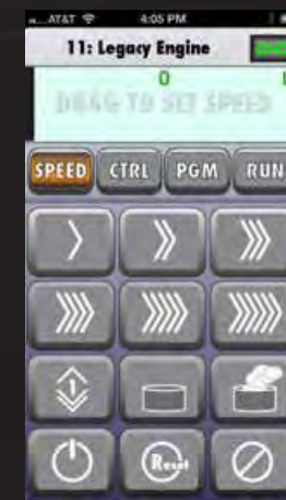
LEFT: Pressing the Xpert button opens the door to three more screens: Speed, Control and Program. Buttons on this screen show preset speeds that get your engine traveling at a specific, repeatable speed. Other Speed page controls include Roll mode, smoke on/off and startup/shutdown keys.
