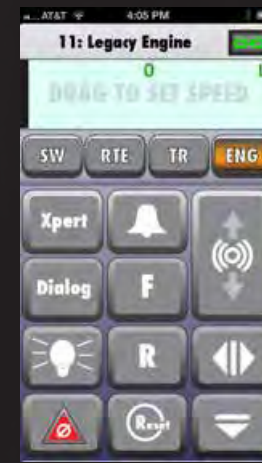
LEFT: The RUN SCREEN will be familiar to users of our LEGACY® CAB-2 hand held remote. The speed graph shows your engine's current speed, and the target speed. Familiar controls, like Bell and Quilling Whistle, Front and Rear Couplers, direction change, and brake are also displayed.
