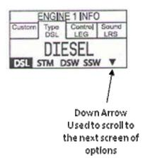
Select the "type" that is specific to the locomotive you are setting up. To select these additional types you can press the key under "Down Arrow". Choose the correct engine type:
