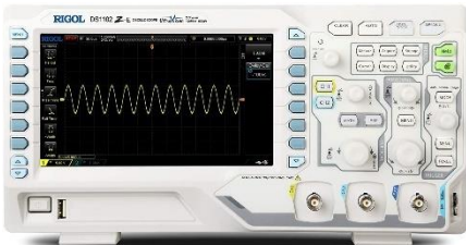
Rigol DS1102Z, 100 MHz, 1 GSa/s, 2 channels. Lowest model in their lineup. About $249.
