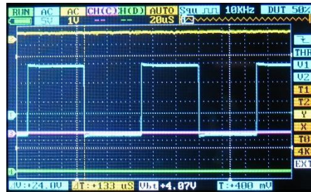
10 kHz 20 Vpp test square wave. Waveform height displaying slightly low.
