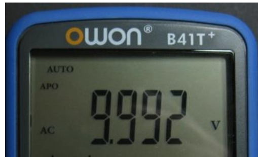
10 kHz 20 Vpp test square wave. 10.000 Vrms is ideal.
