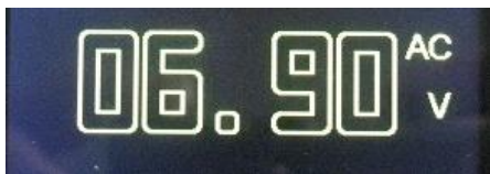
10 kHz 20 Vpp test sine wave. 7.071 V is ideal.
