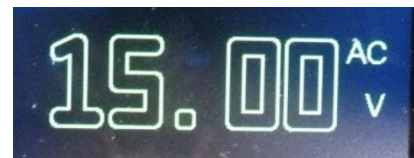
~14 Vrms DCC track voltage.
