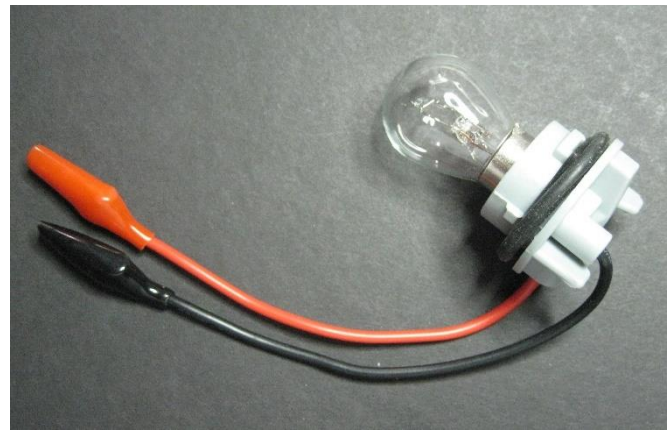
Assembled. (You could solder wires directly to the bulb base, but the socket is convenient for handling.)
