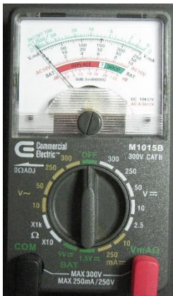
10 kHz 20 Vpp sine. 7.07 Vrms reads 6.3 Vrms
