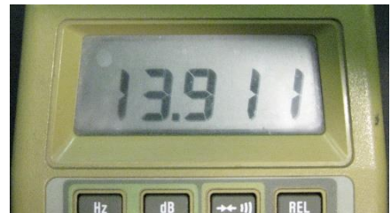
~14 Vrms DCC track voltage reads 13.911 Vrms
