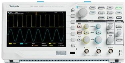
Tektronix TBS1052C, 50 MHz, 1 GSa/s, 2 channels. Lowest model in their lineup. About $504. (Accessories, like probes, extra.)
