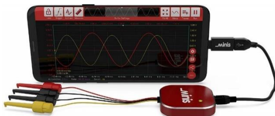
PicoScope 2204A Digital USB Oscilloscope, 10 MHz, 1 GSa/s sampling rate, 2 channels. 5.6 x 3.6 x 0.7 inches. This also has “serial decode” feature and has the DCC protocol built into their software. (Some other scopes also have serial decode, but typically only for industry standard protocols.) About $150.
