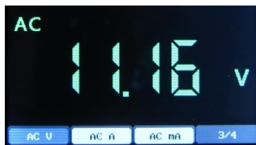
10 kHz 20 Vpp test square wave. 10.000 Vrms is ideal.
