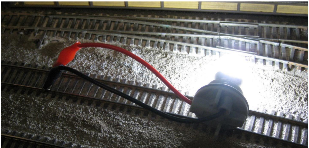
Testing on a layout. Very bright. Only warm to the touch. ~14 Vrms
