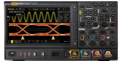
Rigol MSO8204, 2 GHz, 10 GSa/s, 4 channels. Top model in their lineup. About $9,999.
