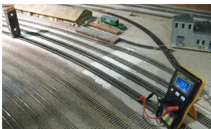
1.67 ohms several feet to the right of the short.
