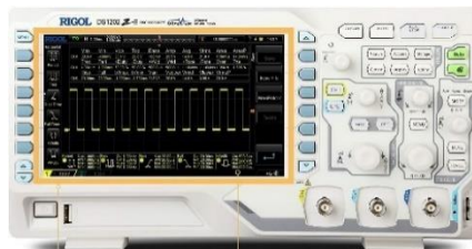
Rigol DS1202Z-E, 200 MHz, 1 GSa/s, 2 channels. Example of a lot more performance for a little more cost. About $299.
