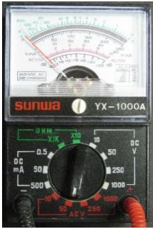
10 kHz 20 Vpp sine. 7.07 Vrms reads 8.0 Vrms.
