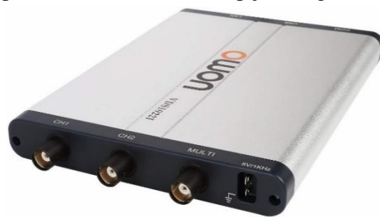
OWON VDS1022I Digital USB Oscilloscope, 25 MHz, 100 MSa/s sampling rate, 2 channels. This has isolation for the USB port so it probably could be used with a computer plugged into the wall and still be isolated. 6.7 x 4.7 x 0.7 inches. About $120.
