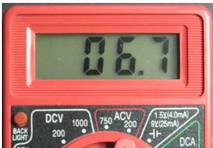
10 kHz 20 Vpp sine wave. 7.07 Vrms is ideal.
