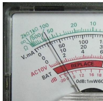
10 kHz 20 Vpp sine. 7.07 Vrms reads 6.3 Vrms
