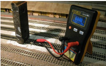
0.040 ohms a couple of inches to the right of the short.
