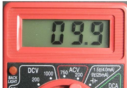
10 kHz 20 Vpp square wave. 10.00 Vrms is ideal.
