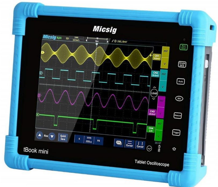
Micsig TO1104 Digital Tablet Oscilloscope, 100 MHz, 1 GSa/s sampling rate, 4 channels. 9.9 x 7.9 x 2.2 inches. About $570.
