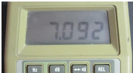
10 kHz 20 Vpp sine wave. 7.071 Vrms is ideal.
