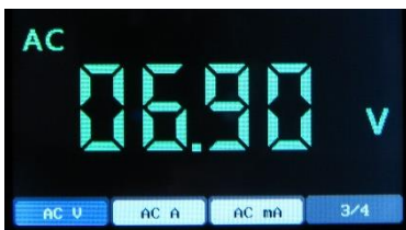
10 kHz 20 Vpp test sine wave. 7.07 Vrms is ideal.
