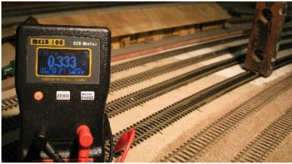
0.333 ohms a couple of feet to the left of the short.
