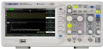
Siglent 1052DL+, 50 MHz, 500 MSa/s, 2 channels. Lowest model in their lineup. About $259.
