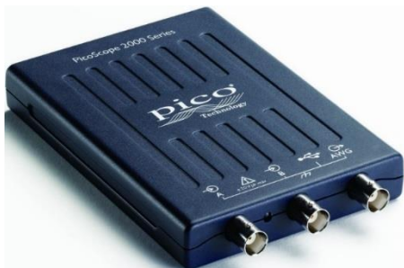
PicoScope 2204A Digital USB Oscilloscope, 10 MHz, 1 GSa/s sampling rate, 2 channels. 5.6 x 3.6 x 0.7 inches. This also has “serial decode” feature and has the DCC protocol built into their software. (Some other scopes also have serial decode, but typically only for industry standard protocols.) About $150.
