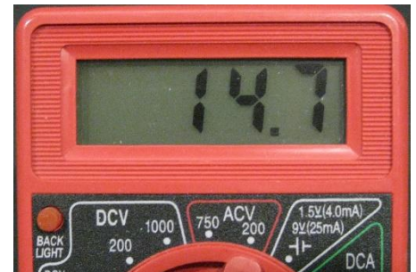
~14 Vrms DCC track voltage reads 14.7 Vrms
