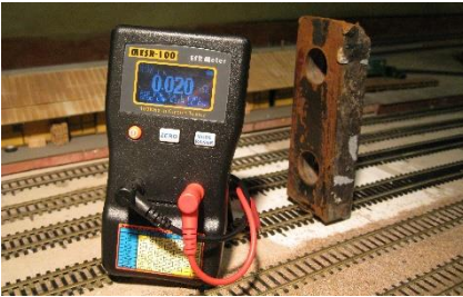
0.020 ohms a couple of inches to the left of the short.
