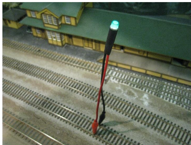
Connected to DCC rails with ~14 Vrms.
