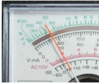
10 kHz 20 Vpp sine. 7.07 Vrms reads 8.0 Vrms.
