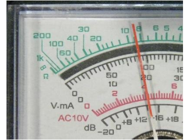
~ 14 Vrms DCC track voltage reads 18.0 Vrms
