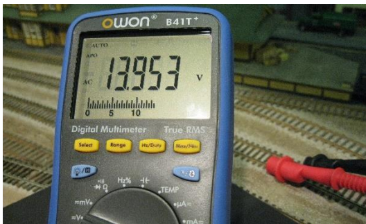
DCC track voltage at ~14 Vrms
