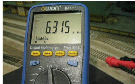
DCC frequency averaging a bit over 6 kHz.
