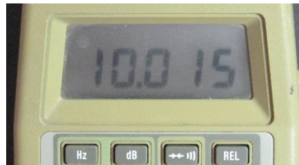
10 kHz 20 Vpp square wave. 10.000 Vrms is ideal.
