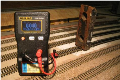
0.040 ohms about 6 inches to the left of the short.
