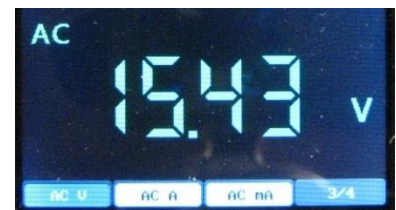
~14 Vrms DCC track voltage.
