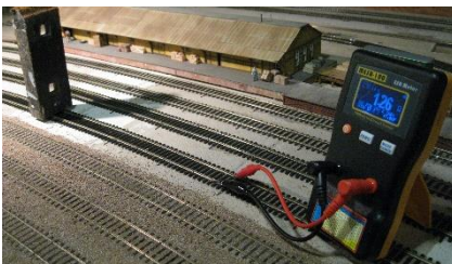
1.126 ohms about a foot to the right of the short.
