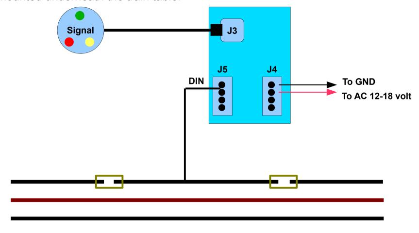
With power connected by this method the signal lights go through a timed sequence
