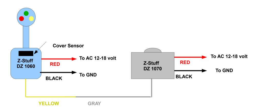
Allows signal to be remotely controlled by the 1070 sensor
