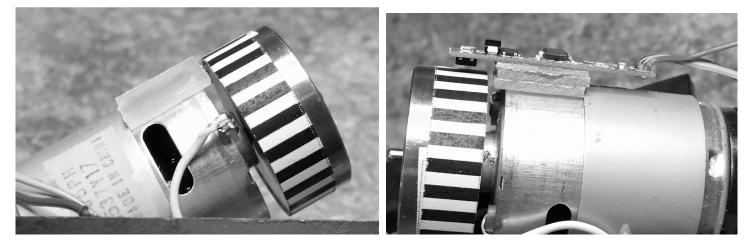
The second installation type is for larger motors, such as the Pittman, found in larger scale steamers. For a large motor install the same curved base is used to mount the C-G to the motor. The difference is that additional spacers are not used as the flywheel is typically smaller than the motor so the sensor will have to be extended to achieve the desired 1mm spacing from the flywheel tach tape. The following illustration shows this type of installation.
