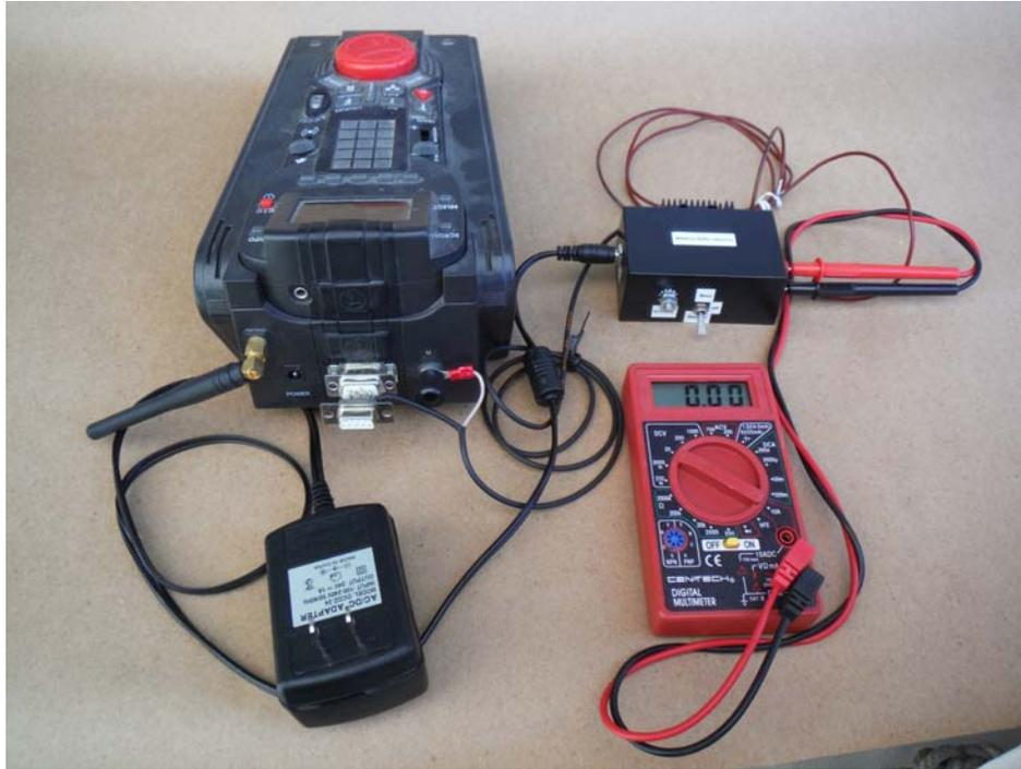
The Buffer/Booster **should not** be mounted adjacent to the TMCC/Legacy Base to keep the Buffer/Booster's higher output signal from interfering with reception of the CAB signals by the Base. The cable attached to the 9-pin DSUB connector provides three feet of range for convenient placement.
