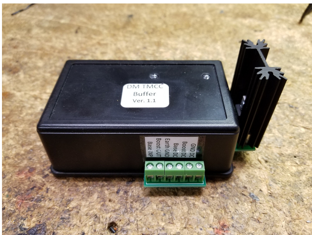
Figure 2 TMCC Buffer Power Amp
