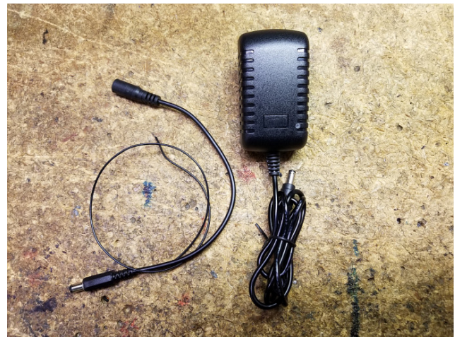
Figure 1 24VDC Power Supply & "earth ground Tether
