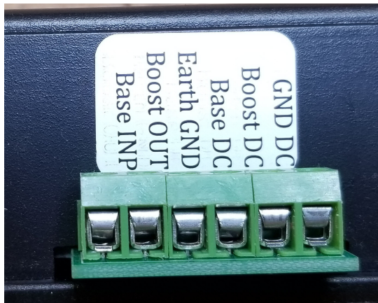
Figure 4 TMCC Buffer Connection Block
