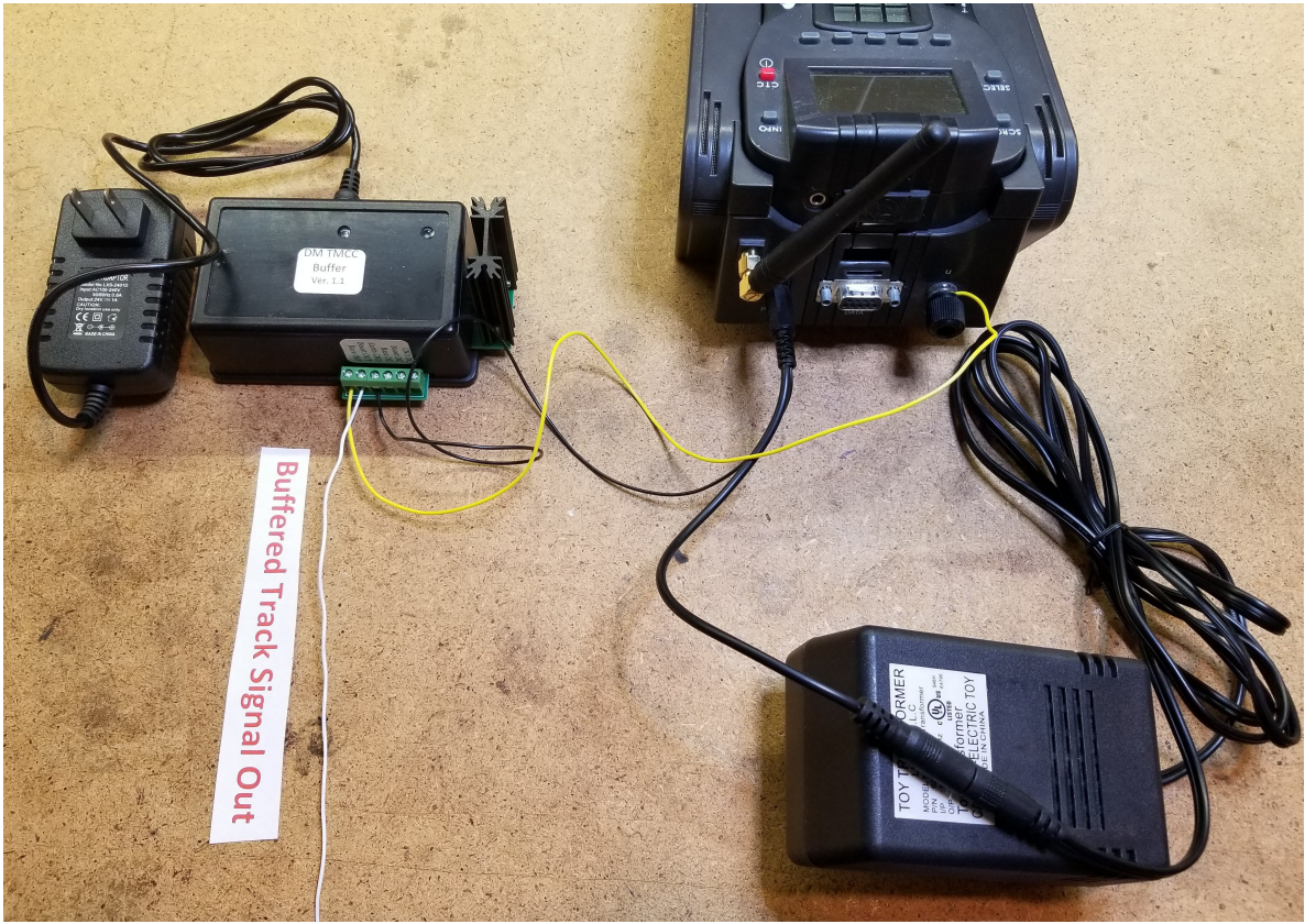
Figure 3 TMCC Buffer Connections
