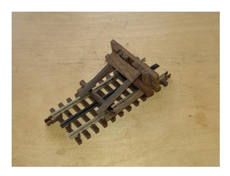
5 – Cut the light panel to length and glue to the top of the angled ties.
