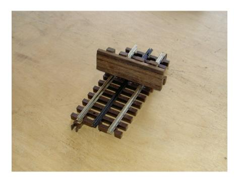
2 –Turn the track so the front of the posts is visible. Cut the bumper wall ties to length and glue together as a sub-assembly then center and glue the sub-assembly to the front of the upright posts on the side opposite the cross member. Be sure the wall assembly rests on the track ties when gluing to the posts.
