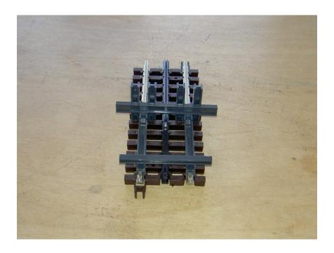
2- Turn the track so the back of the bumper assembly is visible. Cut the B-10 cross member and H-6 back tie to size. Center and glue the B-10 cross member to the top of the H-8 bottom ties and the back face of the posts. Then center and glue the back tie of the top of the H-8 bottom ties about  $\frac{1}{4}$  inch from the back end.
