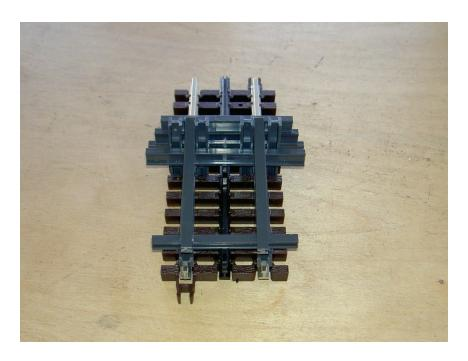
4 – Turn the track once again to the back. Cut the H-6 angle ties to size and glue to the side faces of the two inside posts and to the top of the back tie.
