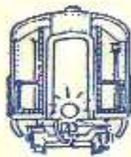
PASSENGER CARS BEING PUSHED AT NIGHT
