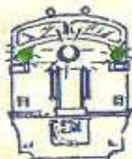
GREEN MARKER LIGHTS MEAN "EXTRA" SECTION FOLLOWING. — LIGHTS LIGHTED AT NIGHT
