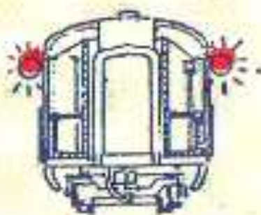
LAST CAR OF PASSENGER TRAIN OR CABOOSE AT NIGHT.
