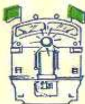
GREEN FLAGS ON FRONT OF ENGINES SHOW "EXTRA" SECTION IS FOLLOWING.
