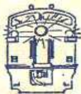
WHITE MARKER LIGHTS MEAN "EXTRA" TRAIN, LIGHTED AT NIGHT.
