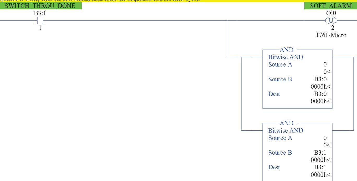
If in manual mode, program is skipped, outputs actually don't matter, but needed only to complete rung.
