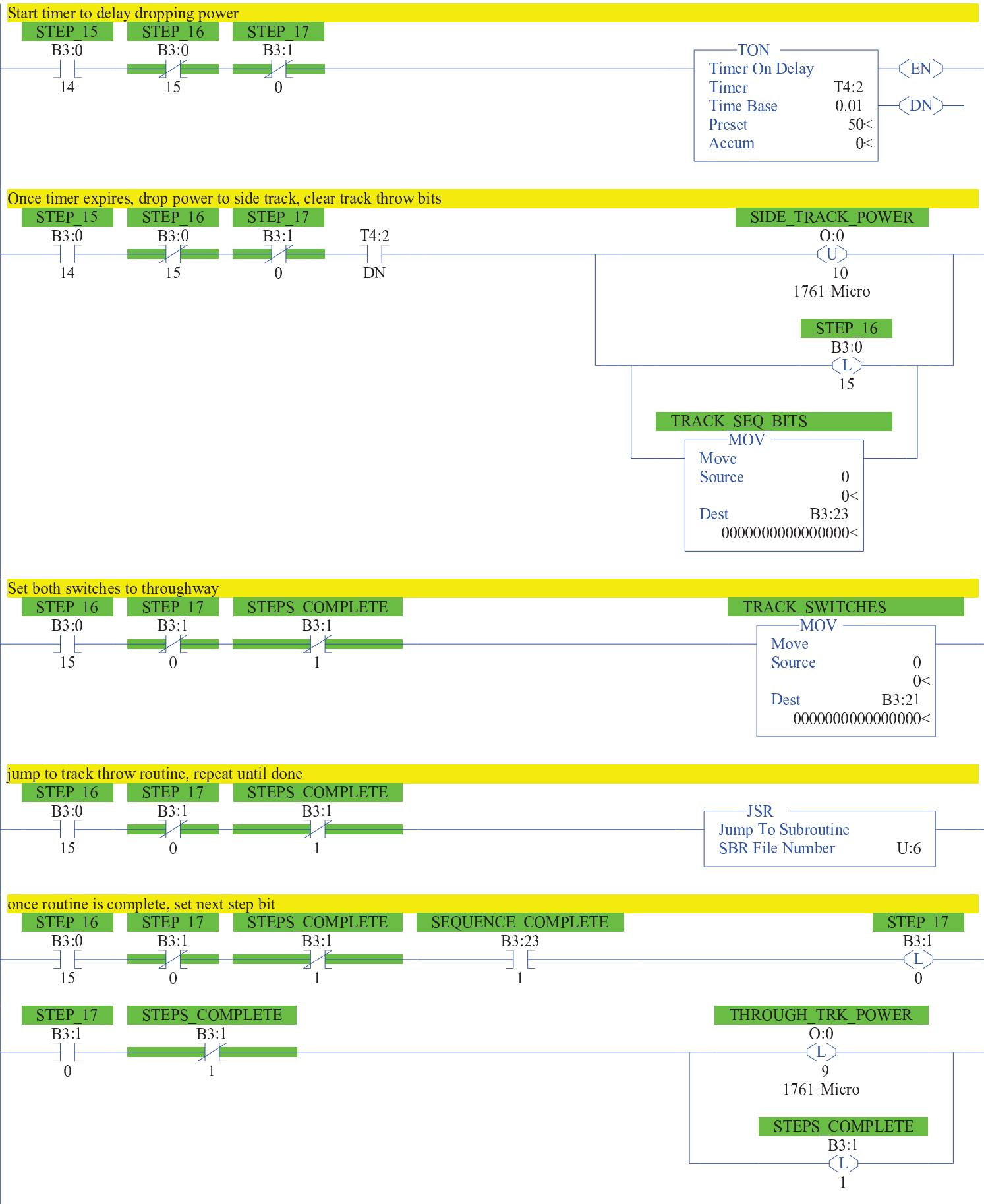
Sequence complete, shut off soft alarm, reset sequence bits for next cycle
