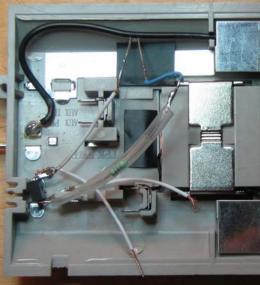
Slide the 3/32" shrink wrap tubing over the blue wire and LED post, so that the two LED posts cannot touch and make electrical contact.
