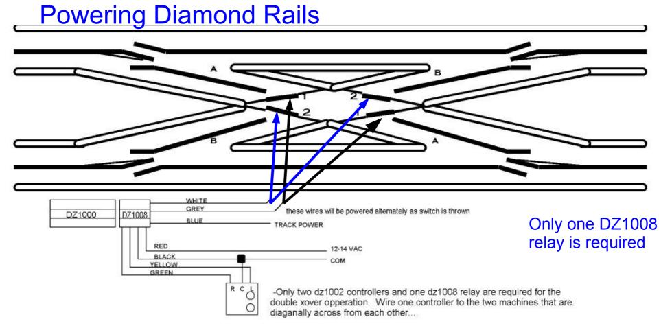
General wire scheme for the DZ 1008 relay (could also use Atlas O Snap Relay) to power rails 1 and 2 in the diamond. When the DZ1008 is connected power to the gray wire is always on unless the relay is activated for route "B". Then the gray wire is turned off and the white wire is turned on. When activated route "A" the gray wire is powered. Having the gray wire powered when the crossover is set for through (straight) is ok since the pick up rollers do not go near the diamond rails.
