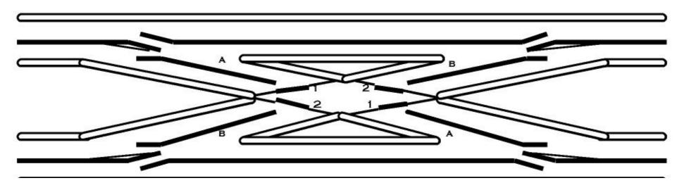
Use the DZ 1008 relay (could also use Atlas O Snap Relay) to power rails 1 and 2 in the diamond. Diamond is non-conductive. All four rails are isolated from each other and normal track. Therefore each rail will need its own wire.
