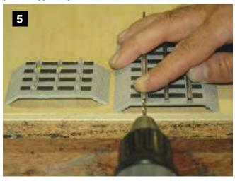
rail. These can be seen if you look at the small section to the left of the track being drilled in **photo 5**. Drill to a depth of at least one half the length of an O-gauge track pin. Be sure to keep the drill against the inside top of the rail and support the rail from above with your finger.
