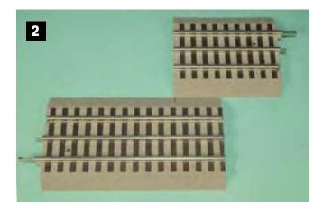
photo 2 and set them so that the measurement from the end of the cut piece to the end of the remaining piece was my desired track length – in this case, 8-1/4 inches. I then marked the larger section at the point where the smaller section ended. This is where the second cut must be made on the larger piece. This is cut in the same manner as before, using the miter box.
