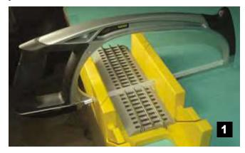
**Photo 1** shows the setup as the sawing proceeds. You must hold the track firmly while sawing. Once you get through the metal rails, the cutting will go quickly. After the first cut was made, I positioned the two pieces as shown in
