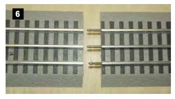
Now place a standard O-gauge track pin into each rail of one of the sections as seen in **photo 6**. You can now press the two sections together for a test fit. If you've been careful, the rail tops and the roadbed will line up properly. For the glue to hold properly, the joint of the two sections of roadbed should touch without any gaps. Next, separate the two sections and place the pins in one section. Sparingly apply Superglue<sup>TM</sup> (cyanoacrylate) to the edge of the roadbed
