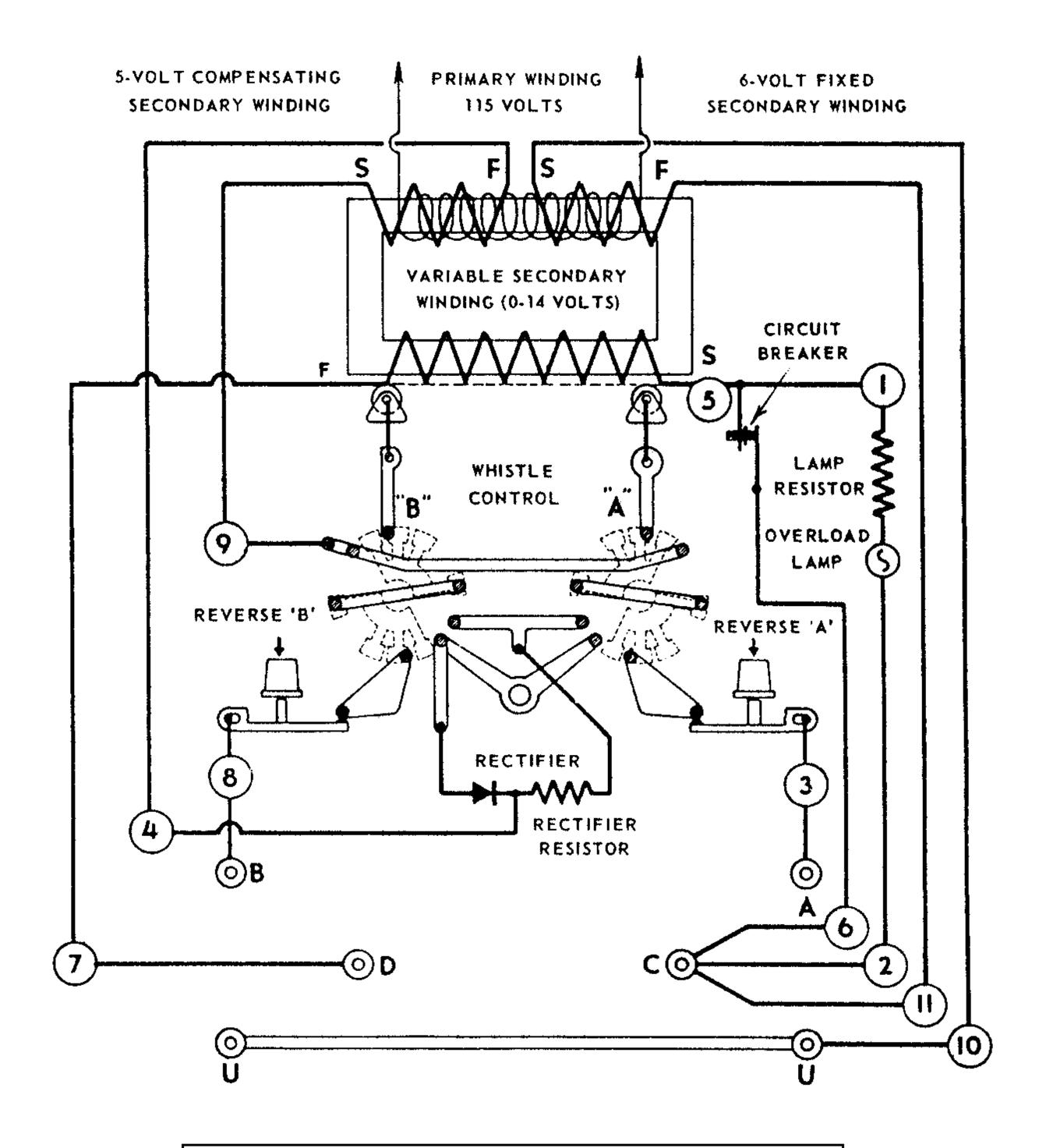
Numbers of leads correspond to those on the pictorial wiring diagram on the opposite page. Letters S and F indicate the start and finish of each winding. Note that the circuit breaker does not protect binding post combinations A-B, B-D and C-U.
