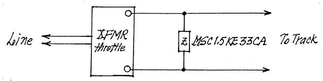
As shown, a maximum sinewave transformer output of 22Vrms can be applied. The whistle/horn button of many traditional Lionel transformers having compensating windings should NOT be used at full throttle, because exceeding this value will result in Zener output clamping and possible loss of protection.
