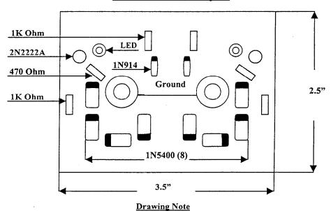
The Ground wire shown is solid bare bus wire and it ties the grounds of the Lamp Screw Bases together on the board.
