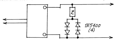
This is still not enough for full-throttle boost insertion, but is the basis for an LED clamp indicator:
